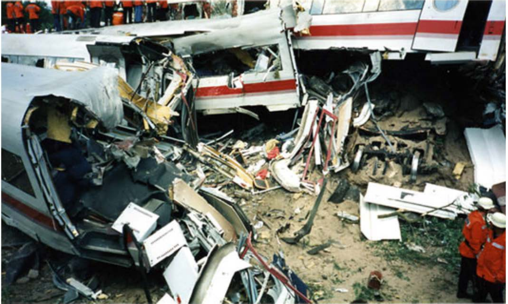
Fig. 1.3 ICE railway accident near Eschede in 1998 as a result of a broken wheel rim
